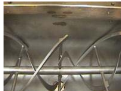
Ribbon mixer after Dry Ice cleaning
