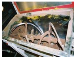
Ribbon mixer before Dry Ice cleaning
