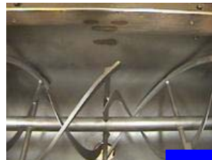
Ribbon mixer after Dry Ice cleaning
