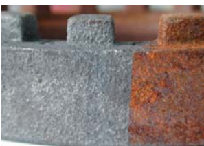
Rusted Metal with Laser Treatment
